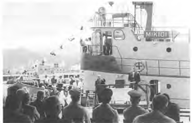
A new ocean-going tug named Mikioi was added to the Young Brothers' fleet in 1960, and then went on to serve Hawaiian Tug & Barge and Dillingham Tug and Barge in the later years. The 106-foot vessel was built by Albina Shipyard and Dillingham Shipyard and was powered with two Fairbanks-Morse engines totaling 2,000-horsepower. Seen here is T.E.W. "Tom" Smith, vice president and operations manager for Hawaiian Tug & Barge, delivering his remarks.
