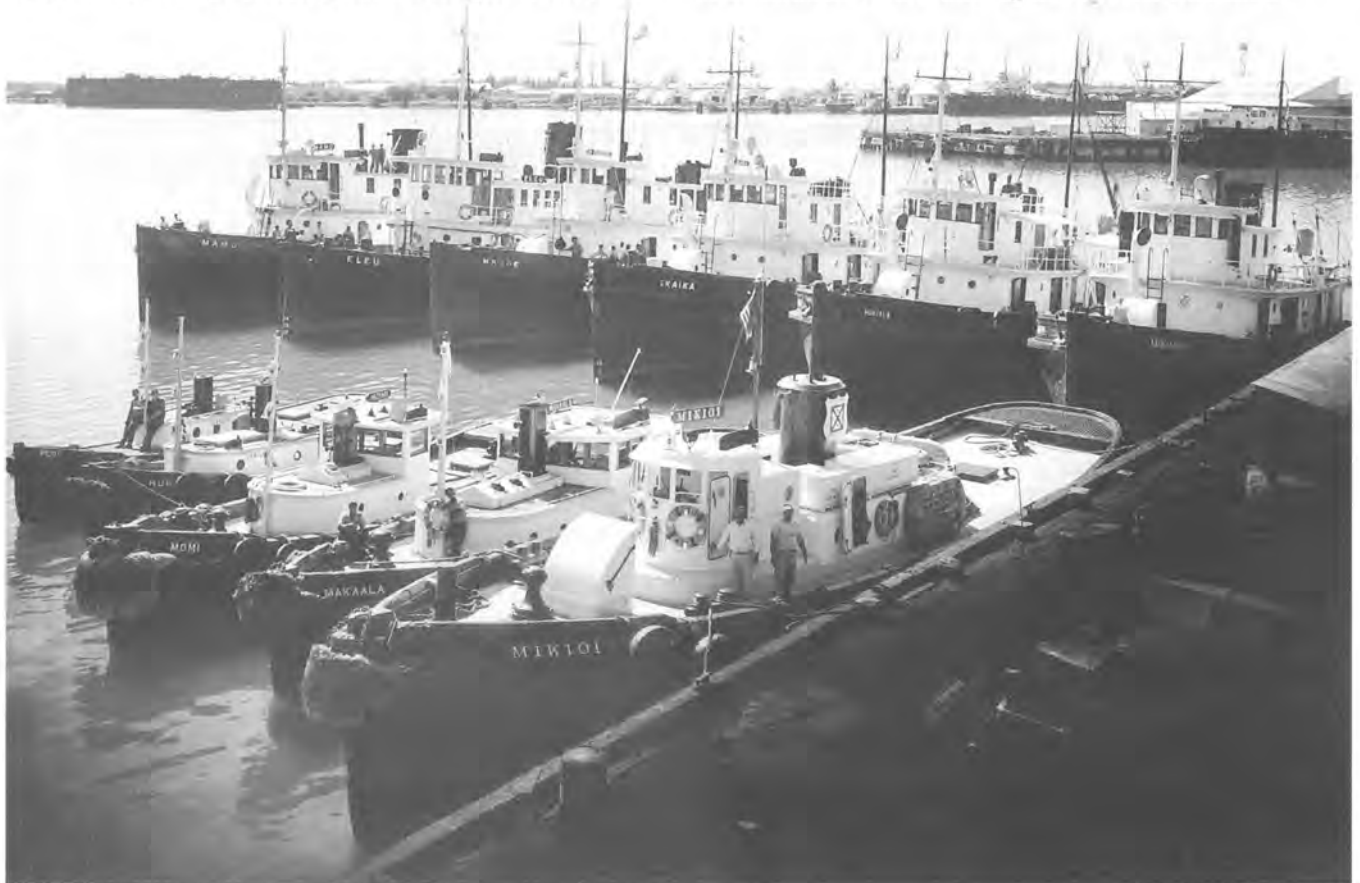
The Young Brothers' fleet at Pier 21 in 1951. The tugboats in the back row were being used for hauling pineapples and towing barges. Pilot, Huki, Momi and Makaala, seen in the front row, were harbor and support tugs used to shift vessels and barges in the harbor, run around doing errands, and take the pilot out to meet ships because the harbor didn't have a pilot boat of its own. Mikioi, seen at front right, would take people out from Piers 9 and 10 to greet passengers on the Lurline and Matsonia. One of the highlights of a voyage to Honolulu would begin just off port. As the incoming passenger liner stopped to pick up the pilot, a troupe of musicians and hula dancers would board a tug to bring the traditional Hawaiian greeting to arriving travelers. Kama'aina would also go aboard to greet arriving friends, and sightseers could even tag along just to experience the thrill of ocean arrivals, for about $5 each. Tugboats in the Young Brothers' fleet, which had been equipped with railings, benches, ladders and life preservers, safely transported the colorful greeting parties. Photo: Hawai'i Maritime Center/Bishop Museum.
