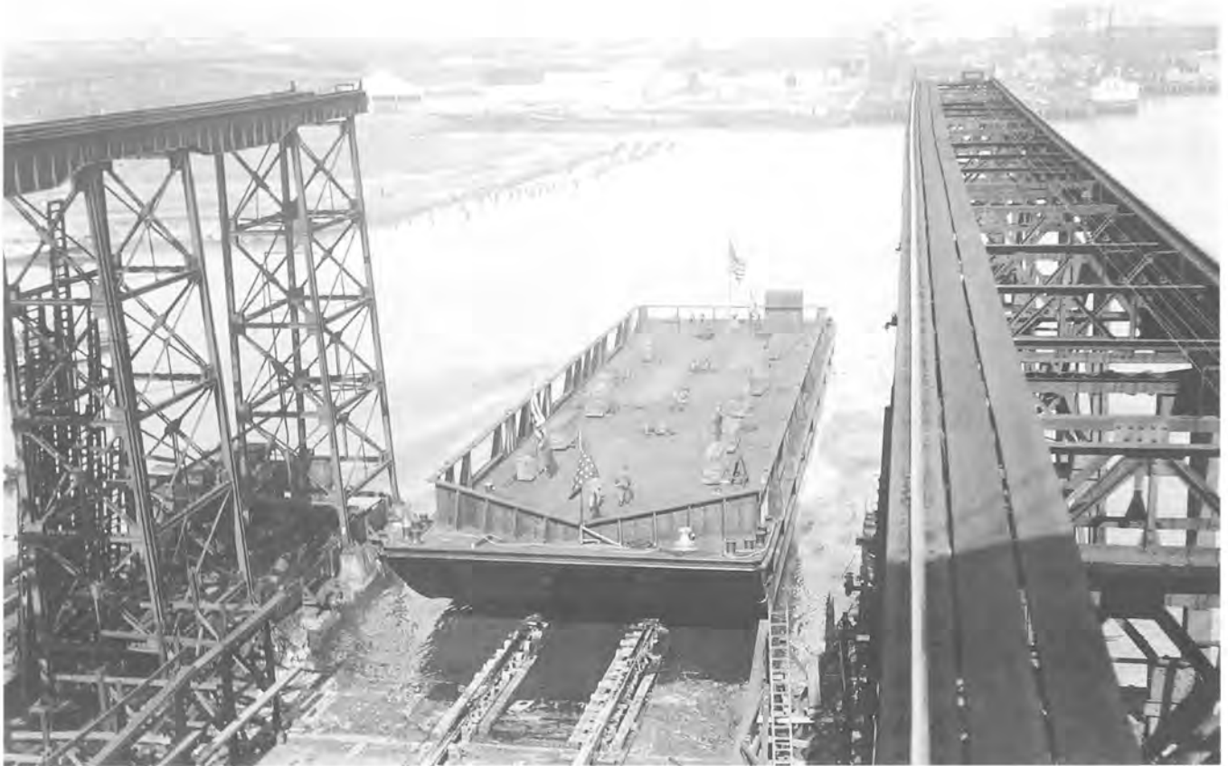
In 1931, the YB-5 was a steel barge built by Union Iron Works in San Francisco at a cost of $65,000. The barge was 175 by 55 feet, and drew twelve feet of water.
