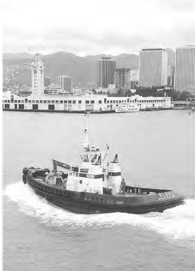
The revolutionary new 2,600-horsepower, Z-drive harbor tug Eleu was designed by Robert Allen Ltd. in Vancouver, B.C. The tug was added to the Hawaiian Tug & Barge fleet in 1990, to increase the company's capabilities, because larger ships were calling on Honolulu that required sophisticated and powerful handling.
