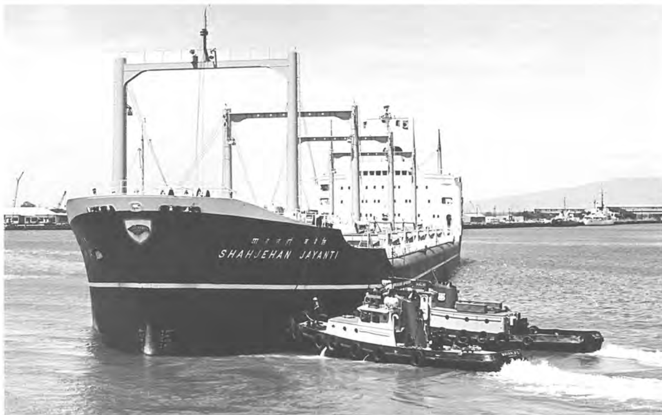
The freighter Shahjehan Jayanti is shifted by tugs Makaala II and Malama. In harbor situations where more power was needed to shift unusually large vessels, the large ocean tugs would assist the harbor tugs.
