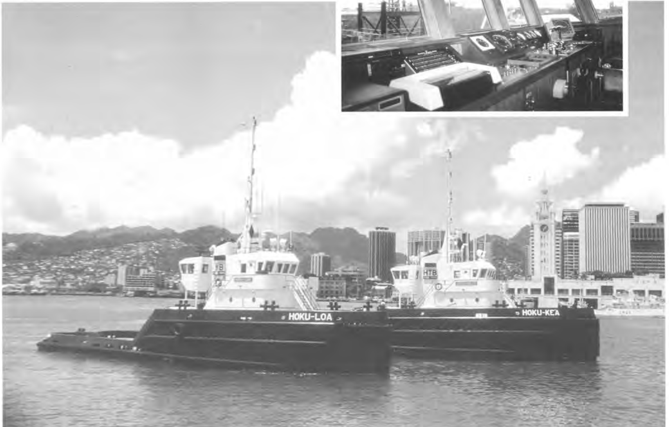
Below: Hoku Loa and Hoku Kea were added to the Hawaiian Tug & Barge/Young Brothers’ fleet in 1991. The 3,900-horsepower twin tugs were built by Bollinger Shipyard in Lockport, Louisiana, and were 108 feet long with a 34-foot beam. Right: Interior of the Hoku Loa.
