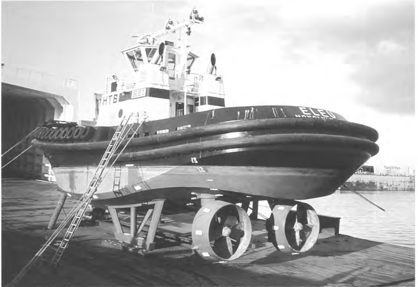
Eleu was launched on January 10, 1990 at the Barbers Point Deep Draft Harbor by floating her off the deck of the partially submerged barge Kamaluhia. Here the Kamaluhia's ballast tanks are being filled, while the Eleu is readied for launch.
