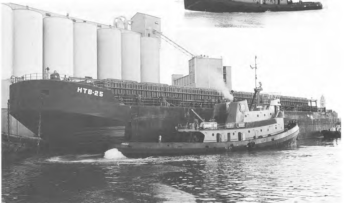
Below: The Mikiona moves alongside HTB-25, a grain and dry bulk cargo barge with a capacity of 8,110 long tons (LT). The flour mill and grain storage tanks (far left) were located at the end of Pier 23. Young Brothers serviced the grain facility for only about two years, until containers started being used. The Mikiona, at right, was launched in 1965, and with its 3,300-horsepower engine, was the largest tug in the Hawaiian Tug & Barge fleet in its day. The tug was 134.5 feet long and had a towing range of 10,000 nautical miles.
