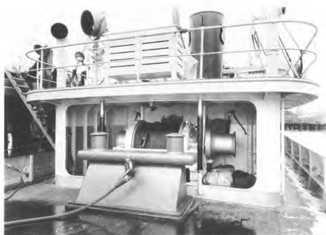
Top: The Mamo is shown nearing completion in Oakland, 1931. The Mamo was 130 feet long with a twenty-eight-foot beam, and had a twelve-foot draft. Above: The towing engine room of the Mamo. Shown is the H-bitt for attaching a second towing line. Instead of two drums, one barge would be attached on the H-bitt, one on the drum.
